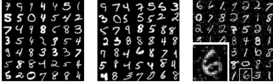
Fig. 1: (Left) 49 digits that the network classified correctly. (Middle) Examples of high-value mistakes generated by our method. They are digits that should be classified correctly, since the images are of the same type as the training images. (Right) Examples of low-value mistakes. They all contain individual pixel-based noise which, though small, is not representative of the types of images the network was designed to recognize.
