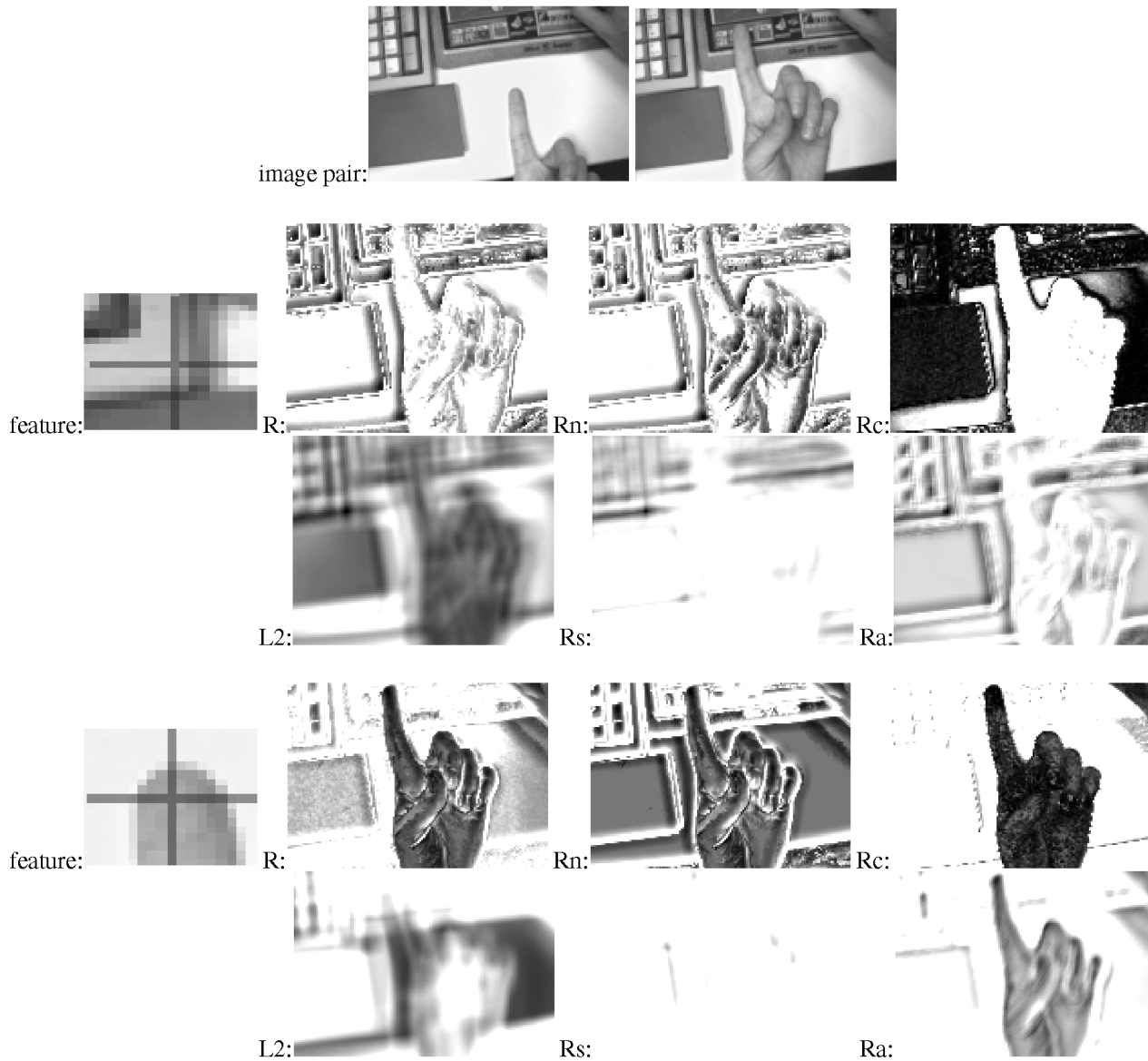
Fig. 3. Correspondence search for two example features. Top row shows an image pair. Left column shows two features selected from left image. Images labeled (R, Rn, Rc, L2, Rs, Ra) show the distance surface of the feature compared to each possible offset in the right image. Images (R, Rn, Rc) are computed using the RCS transform with no smoothing and varying \lambda to illustrate the trade off between neighborhood and color terms (R, Rc, and Rn use \lambda = 0.1, 1.0, 0.0 , respectively). (L2) shows the result using mean-squared-error distance; result with robust norms were qualitatively similar. (Rs) shows the result using an RCS transform ( \lambda = 0.1 ) and isotropic smoothing. (Ra) shows the result using the anisotropic smoothing method described in the text. The corner feature is not near an occlusion boundary, so L2 and RCS methods all have distinct minima at the correct correspondence, and both isotropic and anisotropic smoothing preserve that minima. However, the finger feature is dominated by contrast due to an occlusion boundary and, thus, L2-based methods and isotropic smoothing approaches fail to find the correct correspondence.
